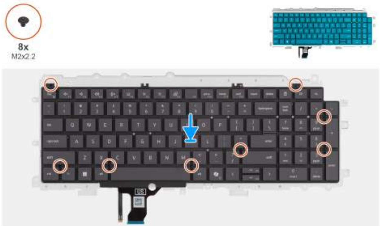
Obrázek 69. Installing the keyboard support plate
