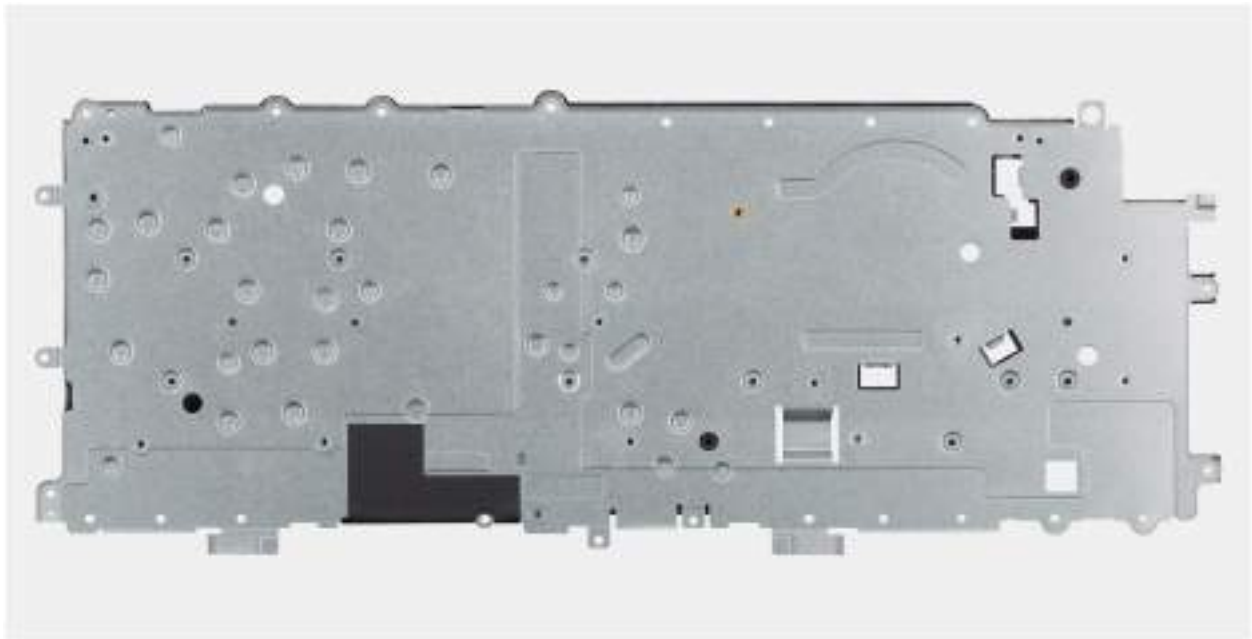
Obrázek 68. Installing the keyboard support plate
