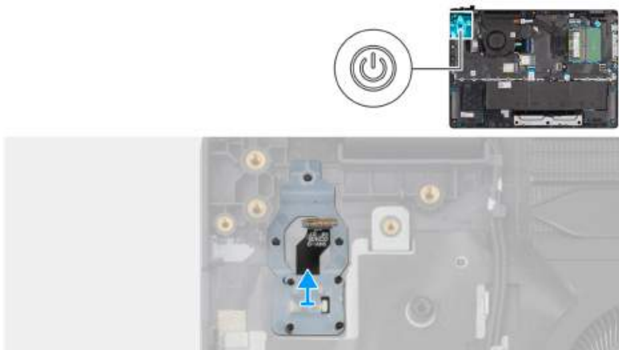
Obrázek 44. Removing the power button with fingerprint reader
