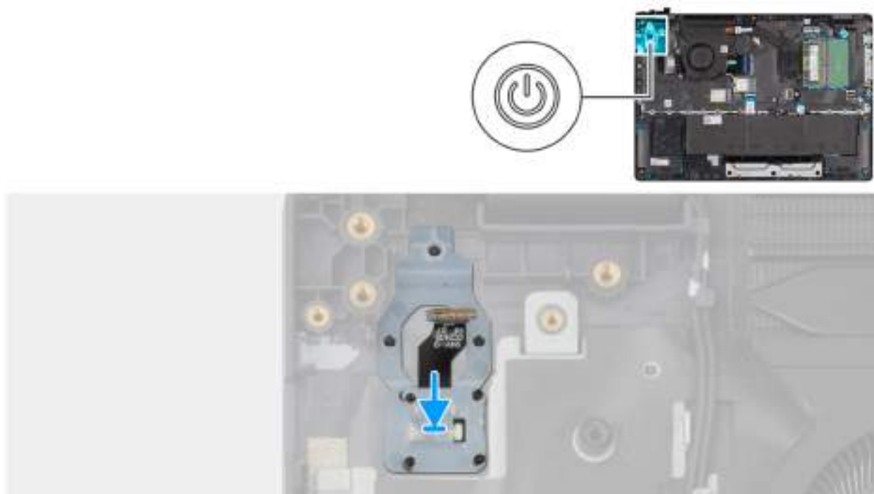
Obrázek 45. Installing the power button with a fingerprint reader
