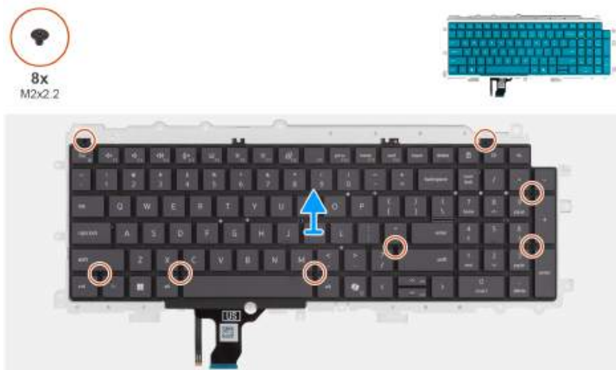
Obrazek 66. Removing the keyboard support plate
